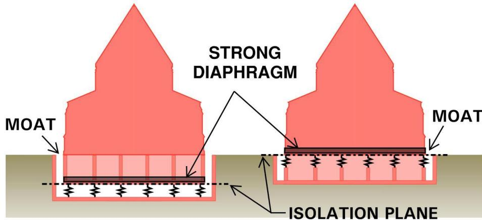
Figure 5. Key requirements of a base isolation scheme
