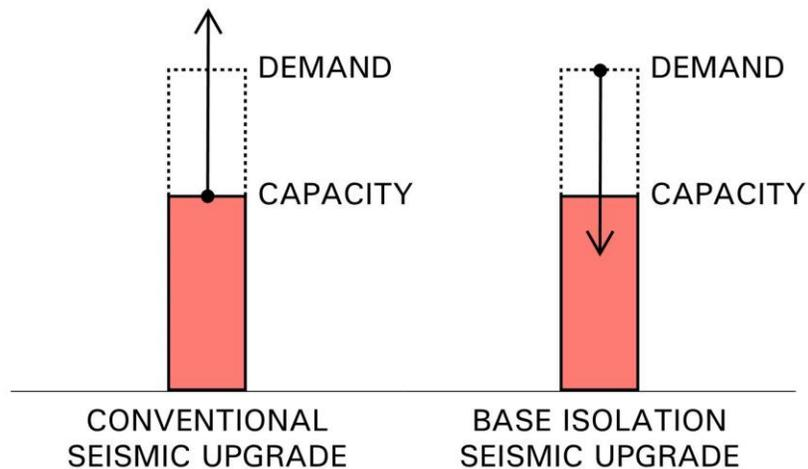
Figure 4. Conceptual difference between a conventional vs. base isolation seismic upgrade approach
